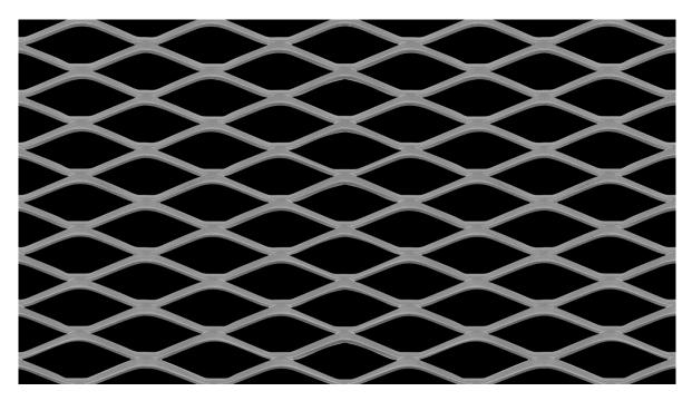
LW Pitch:30.48mmStrand Width:2.36mmSW Pitch:11.72mmThickness:1.20mmWeight:1.28 kg / m2Open Area:59%
